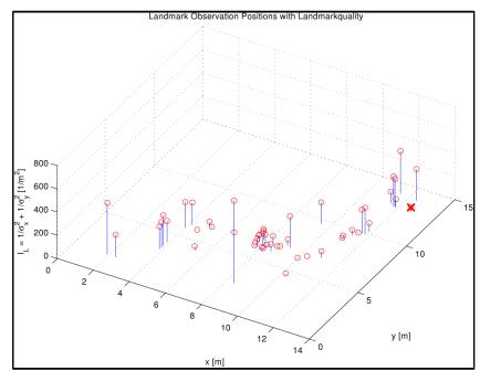
For all landmarks, the estimated observation positions are plotted with the information content on the z-axis. The landmark with the lowest benefit for localization is marked by a red cross. **Hochschule Ulm**
